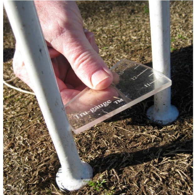
checking hoop width - note that the gauge must be level, and the hoop is measured at half-ball height (as the hoop may not be the same width at all heights)
